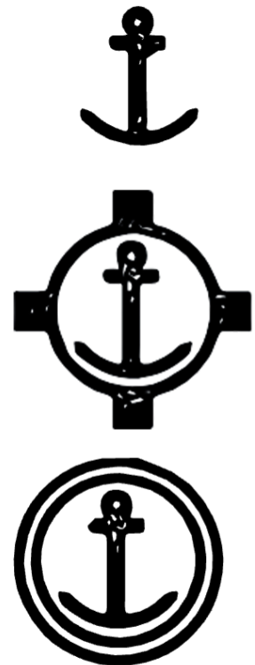
Figure 3. Seaplane base symbology (right graphic). Source: FAA (2004). The top symbol is used to describe a seaplane base that has either no facilities or has incomplete information associated with the base. The middle symbol is used to describe a seaplane base with fuel and services. The bottom symbol is used to describe a military seaplane base with fuel and services.
